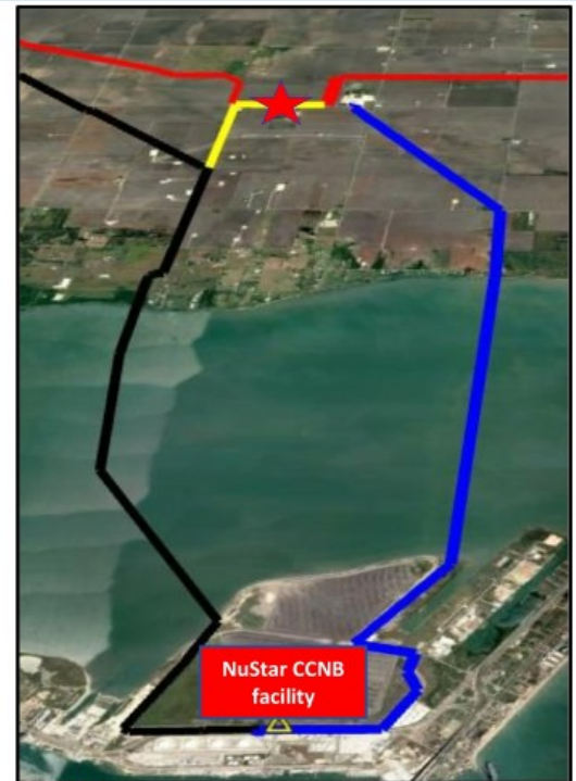
★ NS/PAA Taft connection point — NuStar’s new 30” pipeline — NuStar’s existing 16” pipeline — Plains’ Cactus II pipeline — Early-service connecting pipeline
